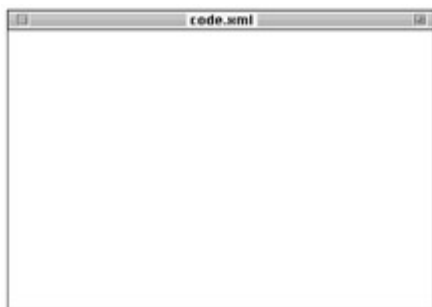
Figure 10.6: [code.xml] If you process an XML document with this style sheet and most basic of root templates, you'll get an empty document. That's what the template in Figure 10.5 says: output two blank lines.
