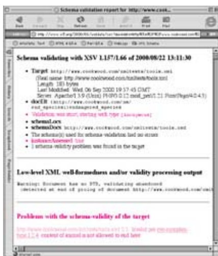
Figure B.4: This time, I only put one name element in my XML file (while requiring at least two in my schema). Consequently, the XSV says my animal element ends too soon.
