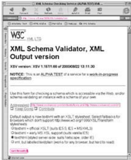
Figure B.3: With the XML Schema Validator (XSV), you type in the URLs of the XML file and Schema file respectively, unless the XML file already references the schema file (and it's available publicly), in which case, just the XML file will suffice. (The files being tested here are tools.xml and tools.xsd, and are at http://www.cook-wood.com/xmltests . Feel free to check them out.
